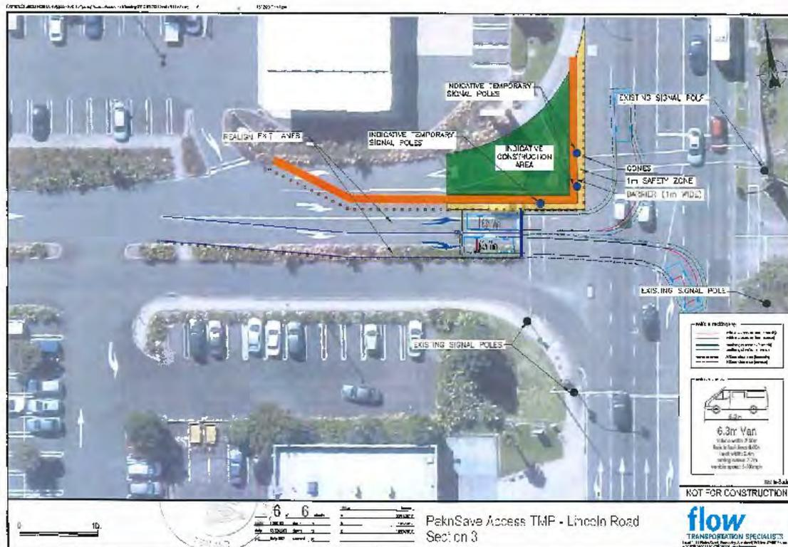
Land requirement plans: these have been included to provide clarification. Blue line shows the extent of the temporary designation for construction (parts of which will be removed post-construction in accordance with Condition 7). Red line shows the permanent designation boundary post-construction).
